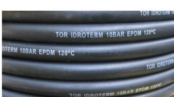
Long length hose with interior and exterior EPDM. Delivery at 10 bar, burst at 30 bar. Working temperature -30°C/+120°C. According to ISO 1307. Hot water / non-corrosive cooling fluids / AdBlue.
