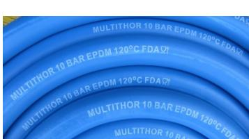
Long length hose with interior and exterior EPDM. Delivery at 10 bar, burst at 30 bar. Working temperature -30°C/+120°C. According to FDA - ISO 1307. Hot water and moderate chemical products.
