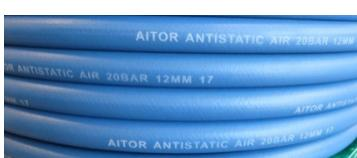
Long length antistatic hose with interior NR/SBR and exterior EPDM/SBR. Delivery at 20 bar, burst at 60 bar. Working temperature -25°C/+80°C. Electric resistance  $1 \times 10^5 \Omega \sim 1 \times 10^6 \Omega$ . According to ISO 1307. Air.
