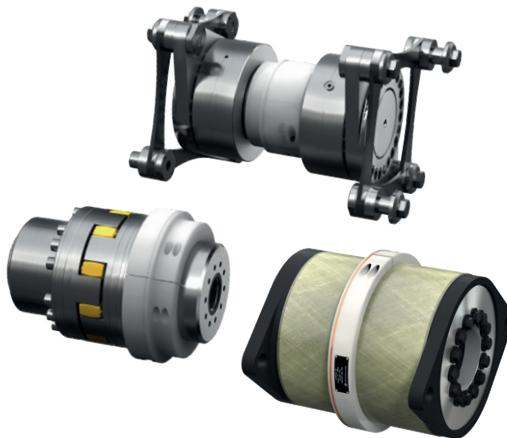
In addition to KTR precision measuring shafts KTR manufactures and calibrates customised measuring shafts for measuring ranges up to 500 kNm. In this context key parameters such as measuring range, size, length and coupling type can be adjusted to the specifications. The torque is measured contactlessly so that bearings are not required.
