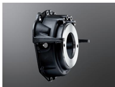
For connecting hydraulic pumps to the diesel engine KTR supplies mounting flanges according to SAE connection dimensions sizes SAE 6 to SAE 1. These flanges are made of steel and EN-GJL-250 for hydraulic pumps with flange connections according to SAE-A, -B, -C, -D and -E as types with 2 and 4 holes.
