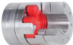
**ROTEX® GS** is a three-part, axial plug-in coupling backlash-free under prestress. It impresses even with critical applications by its backlash-free power transmission, its stiffness which is each adapted to the application and its optimum damping of vibrations. Using this principle provides for significant options of assembly optimizing the assembly times in production.
