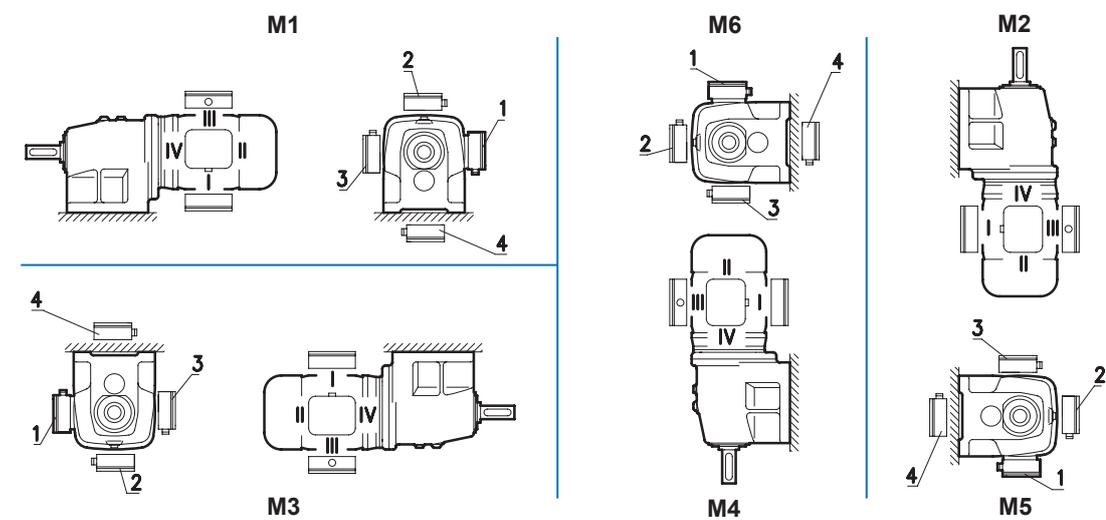
Parallel shaft gear units
