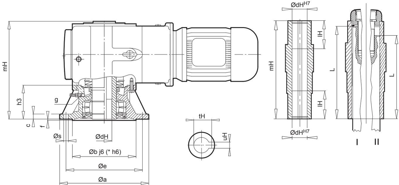
Helical-bevel gear units
