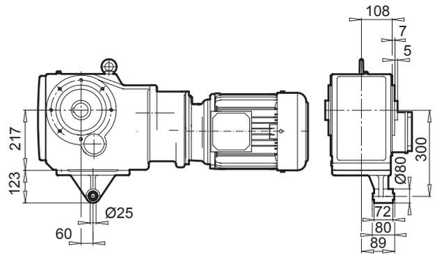
Helical-bevel gear units
