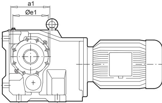
Helical-bevel gear units
