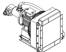
The gear unit oil is drawn in by a pump and flows through a heat exchanger. The oil is cooled by an air stream which is generated by a fan. The oil is then returned to the housing from the heat exchanger. The temperature is controlled by a thermostat. Temperature monitoring is recommended.
