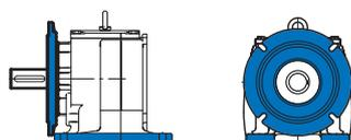
Housing in foot mounted design with Flange B5,
