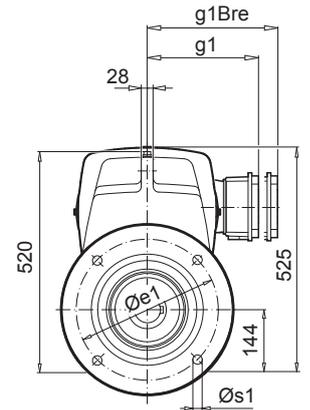
Parallel shaft gear units
