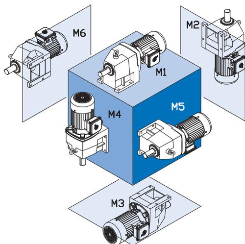
Parallel shaft gear units
