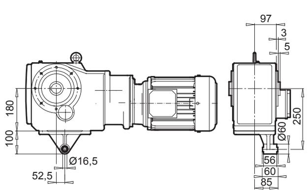
Helical-bevel gear units
