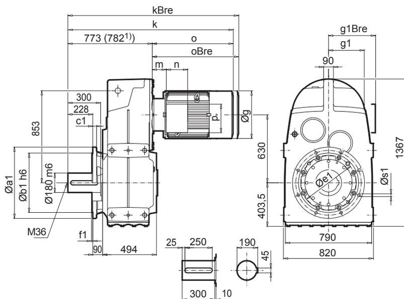
Parallel shaft gear units
