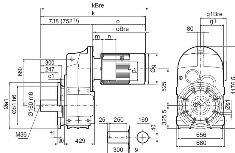
Parallel shaft gear units
