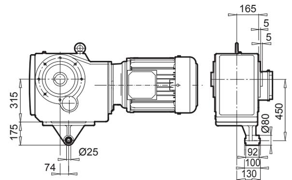
Helical-bevel gear units
