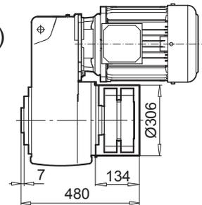
Parallel shaft gear units
