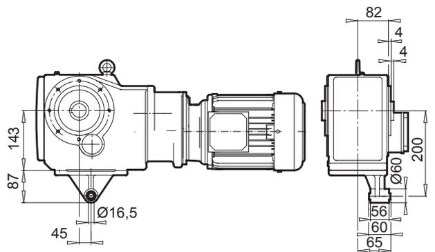
Helical-bevel gear units
