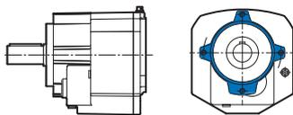
Housing in flange mounted design with Flange B14
