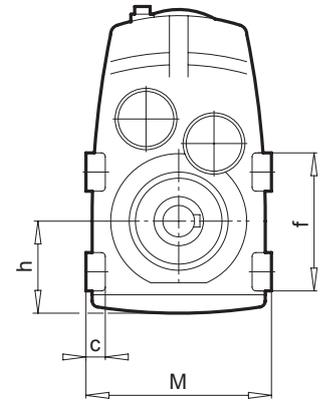
Parallel shaft gear units
