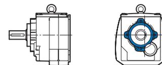
Housing in flange mounted design with Flange B14,
