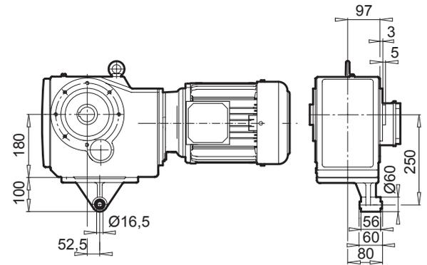
Helical-bevel gear units
