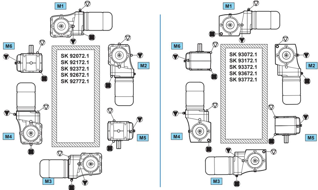
For the NORD gear unit series SK 92x72.1 it should be noted that for structural reasons, the shutter or venting screw can only be mounted on the side opposite to the motor and protrudes beyond the footprint.
