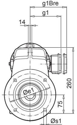
Parallel shaft gear units
