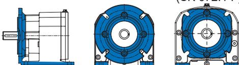
Housing in foot mounted design with Flange B5
